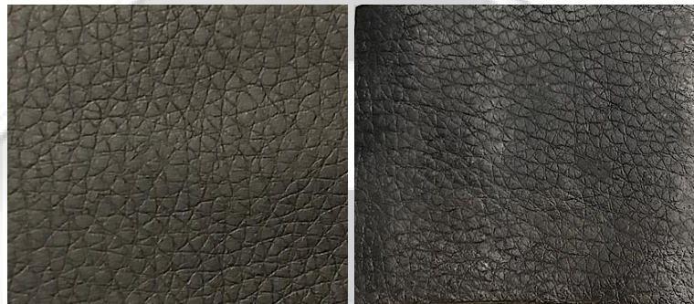
Photo 2: PRIME 2.0 PU Leather Left: As received on 26 Mar 2019 Right: After Immersion Test and Chamber Conditioning
