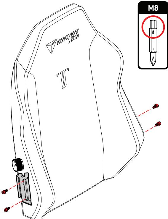
**05** Slide the backrest bracket on the right down onto the right recline bracket until it comes to a stop. Insert the M8 screws (from Step 4) and screw them in halfway.
