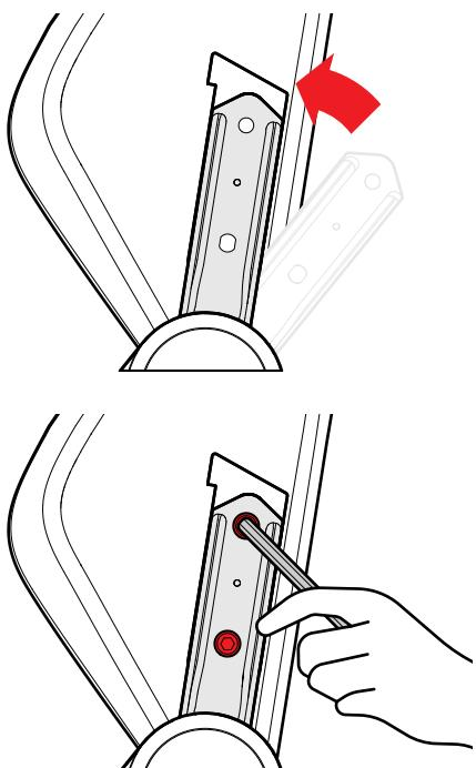
**07** Install the magnetic side covers by aligning them on top of the backrest brackets on both sides. They will magnetically snap into place.
