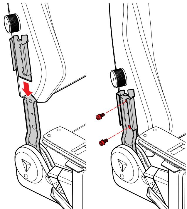
**06** Push the left recline bracket up to align with the screw holes on the left of the backrest. Insert the M8 screws and fully tighten all 4 screws on both sides with the long allen key.
