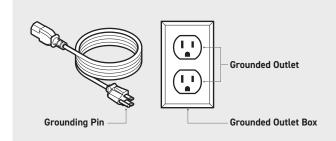
**WARNING:** This product is for use on a nominal 100-240 volt circuit and has a grounding plug. Use only the cord provided. Make sure that the product is connected to an outlet having the same configuration as the plug. Do not modify the plug provided with the product. No adapters are to be used with this product. Keep cord away from heated surfaces.
