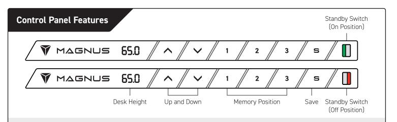
**STANDBY SWITCH.** The Control Panel can be turned off to prevent accidental activation or movement of the desk. Slide the switch to the right to turn it on. Slide it to the left to turn it off.
